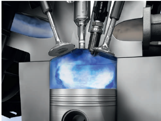
Figure 2.221 New petrol/gasoline injection system
